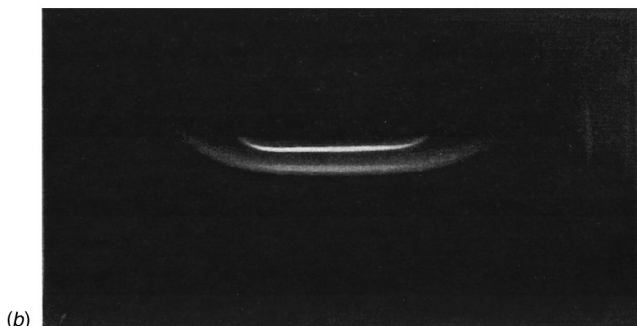
Fig. 1 (a) Schematic diagram of a two-stage flame of ethane in counterflowing streams; (b) a photograph of the flame sketched above.
